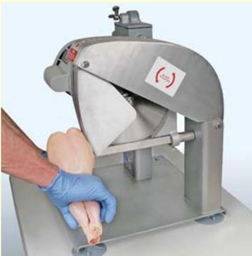
The operator's left hand holds and pulls both wings (together) down over the apex precision guide bar as shown, exposing the wing knuckle joints. Operator keeps both hands below the precision guide cutting bar.
