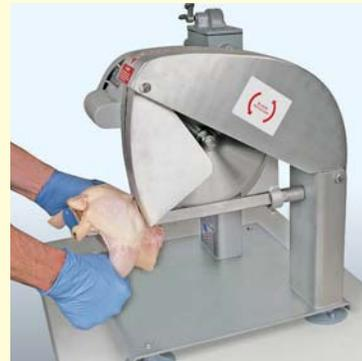
Holding one drumstick in each hand, position right thigh and drumstick over the apex guide bar, keeping both hands below the guide bar as shown. Bird is now poised for removal of drumstick and thigh.
